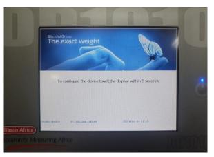
2. To enter the system setup, touch the screen at start-up within five seconds.
